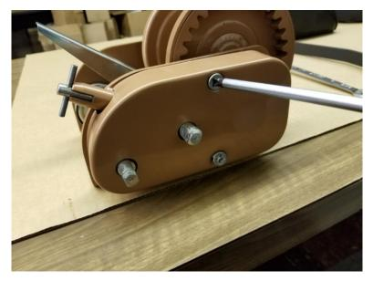
1. Remove gear cover screws (S) using a large Phillips screwdriver. Then pull gear cover (C) off of winch in order to expose gears and ratchet plunger housing.
