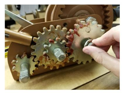
9. Place the 20 tooth gear (N) back onto short drive shaft (M) with the gear breakout side (flat side) facing away from the base. Then place washer (O) and screw (P) in middle hole and tighten in clockwise direction. 20 tooth gear and intermediate drive shaft should have suitable gear mesh and the winch should operate normally.
