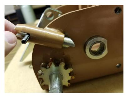
6. Now it is time to reassemble the components. This process is simply working back through the steps above. Push the new ratchet plunger and spring (V &W) up into the ratchet housing from the bottom of the housing, and then tap the roll pin (U) into the plunger from the side as shown in the picture above.
