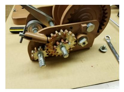
3. At this point, the winch should look like the picture above. The intermediate drive shaft (DD) must be removed next. This can be achieved by removing two retaining rings (BB & KK) from the shaft using a straight screwdriver or snap ring pliers. Once these rings are removed, the shaft should be able to be pulled out of the winch in order to access the bottom of the ratchet plunger housing.
