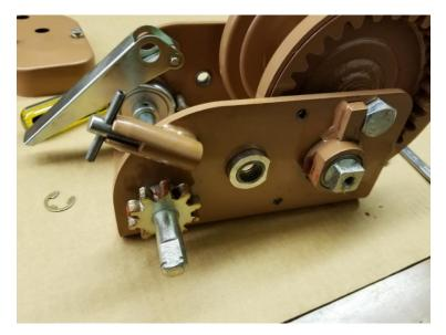
4. Turn the ratchet plunger to the engaged position (roll pin turned sideways and plunger sticking out). Using a 5/32" diameter pin-removal punch, remove the roll pin from the ratchet plunger. The ratchet plunger (V) and spring (W) can now be removed from the bottom of the housing.
