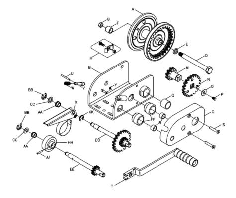
Replacement of the ratchet plunger (V), ratchet spring (W), and roll pin (U), will require some disassembly. The gear cover (C), 20 tooth gear (N), and intermediate drive shaft (DD) will need to be removed in order to access the bottom of the ratchet plunger housing. This will require a large Phillips screwdriver, a 9/16" wrench (for screw (P) removal), a straight screwdriver or snap-ring pliers (for retaining ring removal), and a 5/32" diameter pin-removal punch (for roll pin (U)).
