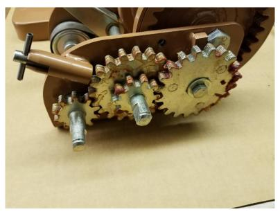
10. The winch should now look like the picture above. The gear cover (C) can now be placed back onto the winch, and can be tightened down by its two screws (S).
