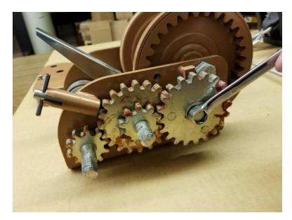
2. Using a 9/16" wrench, remove screw (P) and washer (O) from middle of 20 tooth gear (N) by loosening the screw counterclockwise. This process can be accomplished easier by pressing the Brake Handle Assy (X) down with one hand while loosening the screw with the other hand, jamming a screwdriver in between the gears, or, if the ratchet plunger still has some spring pressure, allowing the plunger to lock the gears. Then remove the 20 tooth gear and set it aside.
